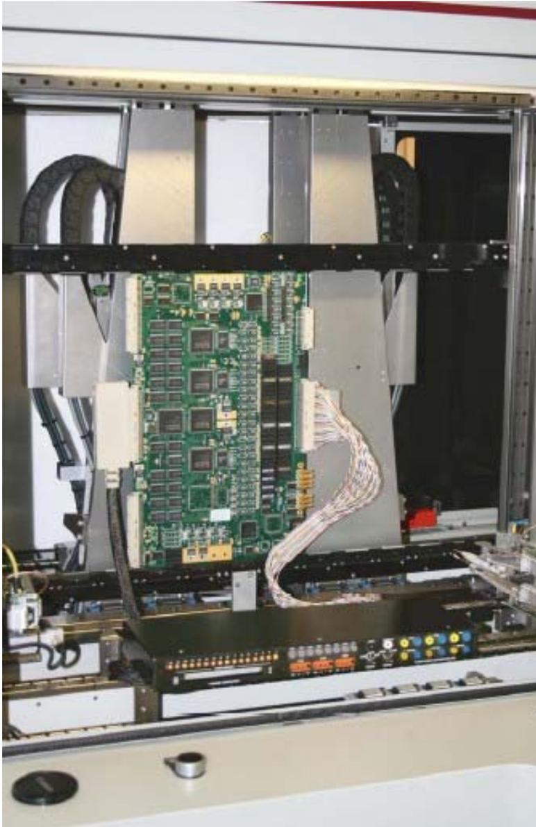
**Figure 6:** Once the GND and VCC inputs have been identified on the UUT, we can connect a cable with supply voltages and the PWMON procedure can be started to detect possible digital faults on the ICs.
