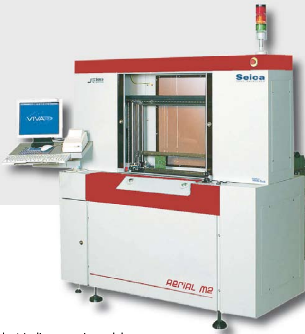
ATE flying probes Aerial M2
