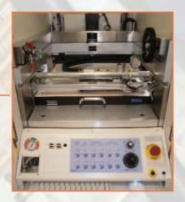
Configuration offers a completely automated solution via an integrated, SMEMA-compatible transport system, allowing completely automatic board handling and easy integration into high volume production lines. Configurable as ICT, pre-functional, functional and combinational
